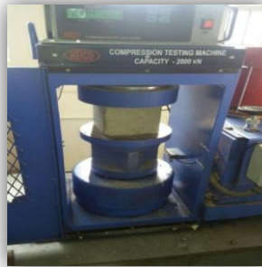
Figure 5: Split Tensile Test
