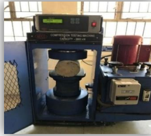
Figure 4: Compressive Strength Test
